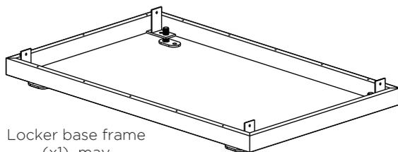
Locker base frame (x1) may or may not have levelling feet installed)
