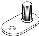
Adjustable levelling foot (x4 per base frame, may already be installed in)
